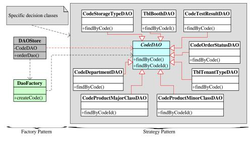
FIGURE 4 Class diagram of database accessing middleware
