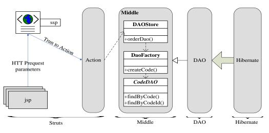
FIGURE 3. Structure of Database Accessing Middleware
