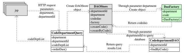
FIGURE 7 Process of applying database accessing middleware
